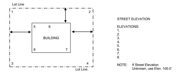
Direction of slope from building to lot lines are as per diagram.
